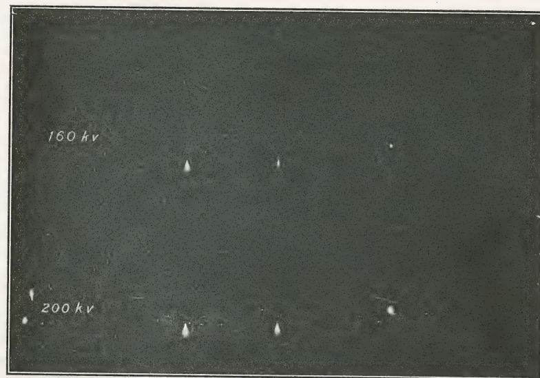
FIG. 66.—Corona on a No. 3/0 line cable. Dry.
