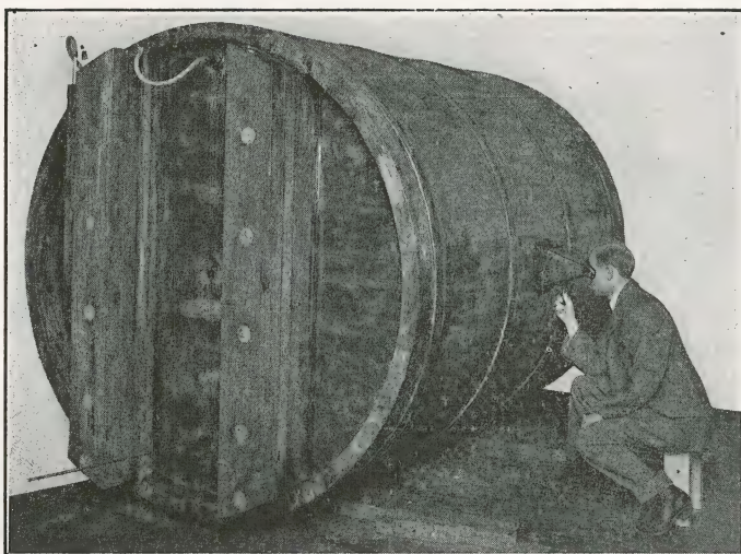
FIG. 104.—Cask for the study of the variation of spark-over and corona voltages with air pressure.
