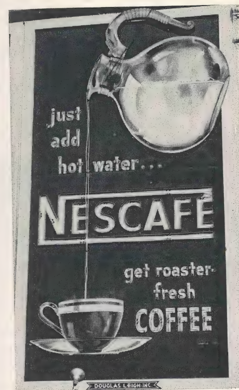
FIG. 12-8. A spectacular luminous-tube sign. Two rows of tubing running vertically and alternating by rapid flasher action produce the effect of coffee pouring into the cup. Smoke from the cup is produced by a special smoke generator.
