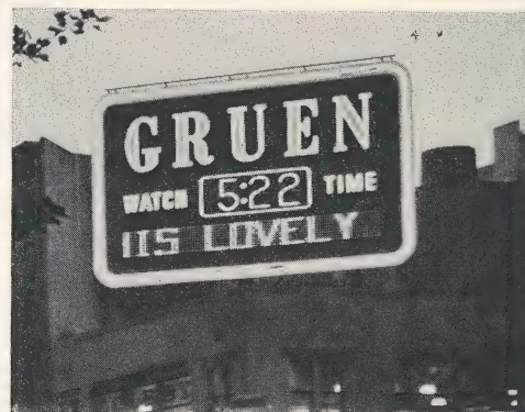
FIG. 12-7. A neon sign combined with a jump clock for direct reading of time in hours and minutes.
