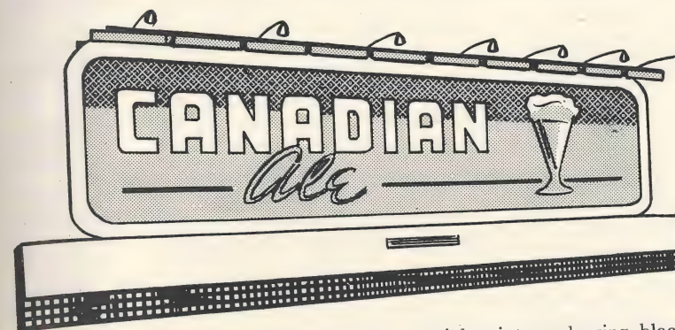
FIG. 15-3. A bulletin board painted with special paints and using black-light lamps and spotlights. The black-light lamps are lit all the time, while the spotlights flash on and off, producing distinct changes in appearance and wording.
