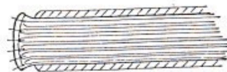
FRENCH JOINT with boards attached to outside of sewing support
