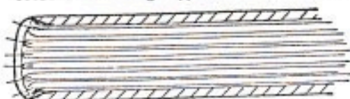
TIGHT JOINT with boards attached to inside of sewing support
