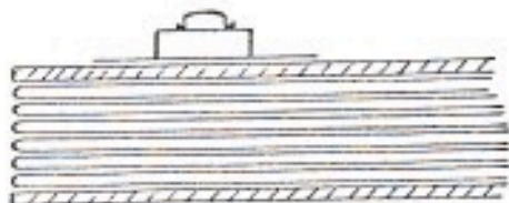
THICKNESS OF SECTIONS PLUS BOARDS under light pressure (swelling from sewing to equal thickness of boards)
