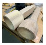
4) Replaced on Lathe - rough shaped as handle. 'Between Centers'
