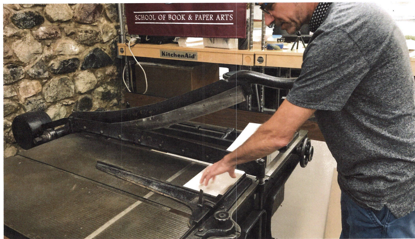
Tom Hollander demonstrates on a 121-year-old board shear (Photo: Meredith Bruckner)
