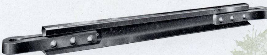
Connecting link or reach for coupling cars to the Clyde Decker Loader.
