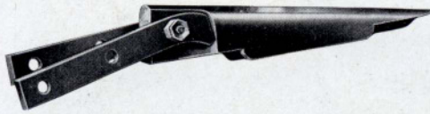
Manganese steel point on shoe used on the end of the rail inclines on Clyde Decker Loader.
