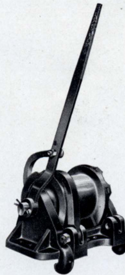
Hand Ratchet drum used on Clyde loaders for taking up slack in the side guying lines when using the machine for skidding.
