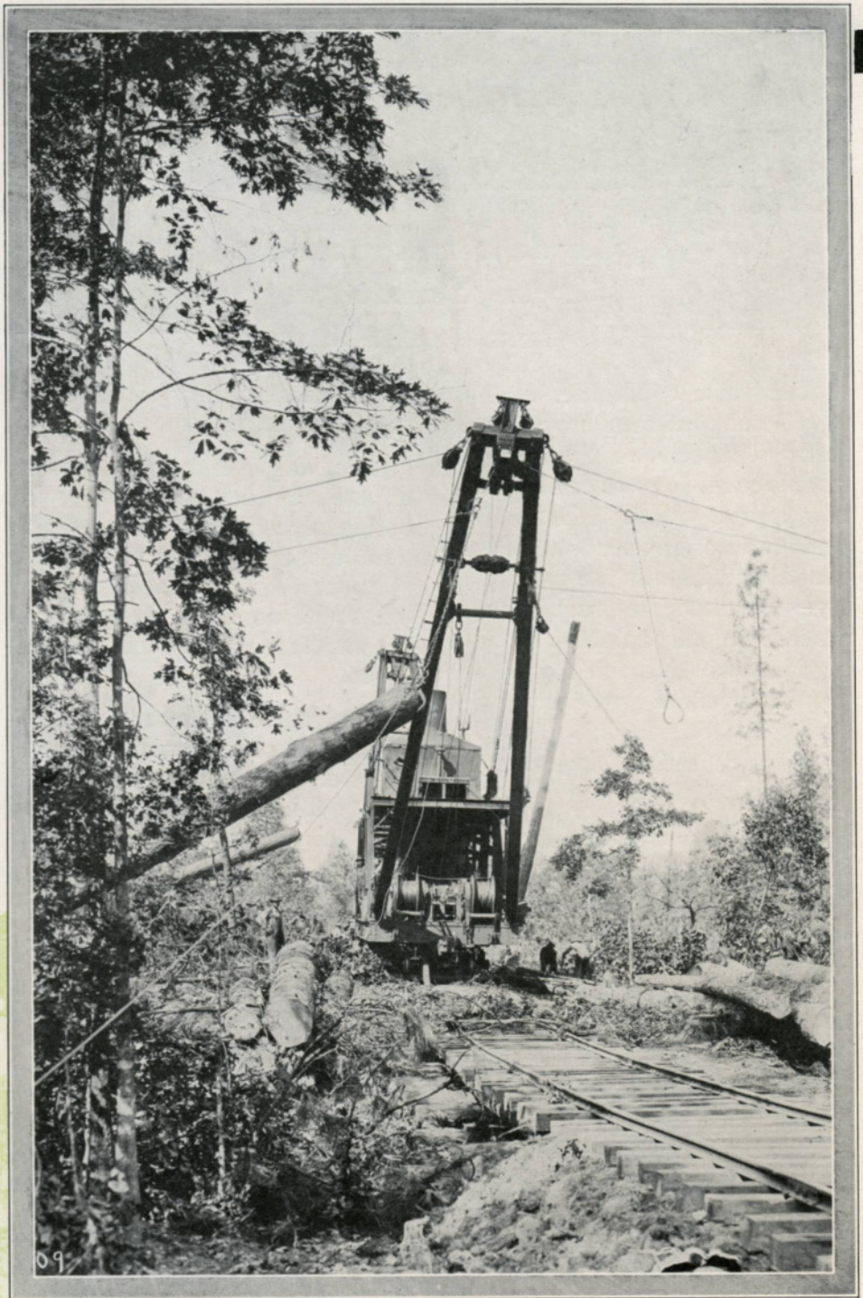
Clyde Four-Line Skidder With Cable Outhaul.
