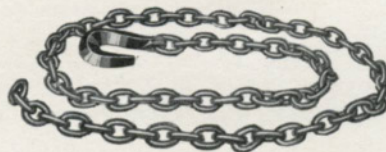
Anchor Chain: \frac{3}{4} -inch chain 10 feet long, with grab hook one end. For attaching outhaul block to tree or stump.
