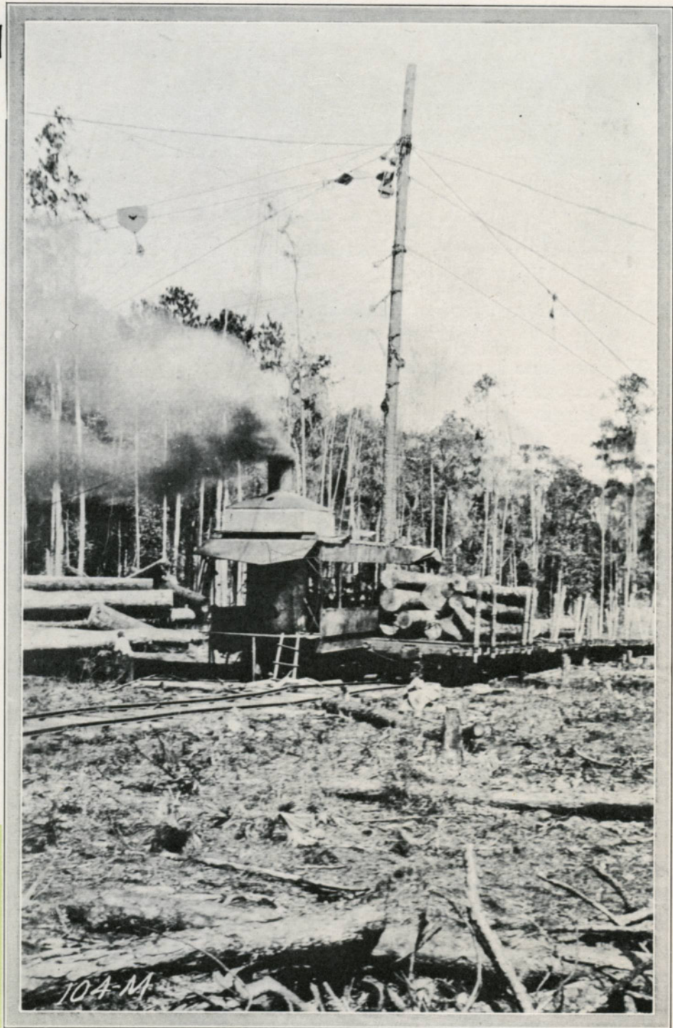
Clyde Cableway Skidder and Loader for Tree Rigging.
