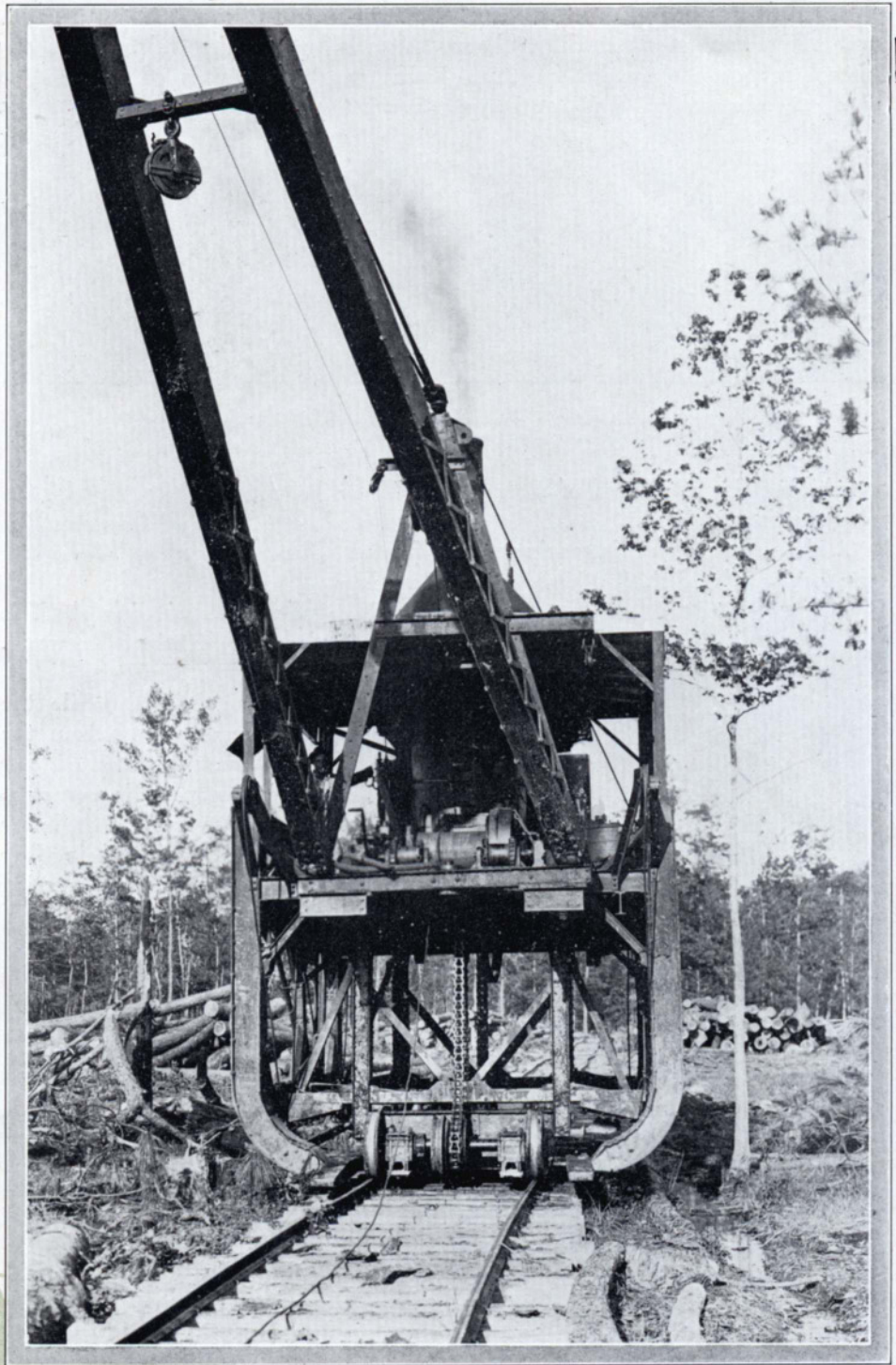
McGiffert Loader, swing boom, 4-wheel trucks, with trucks down, resting on wheels for moving along the track.
