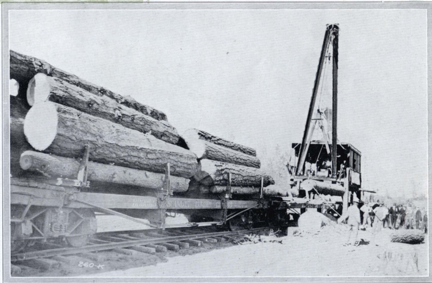
McGiffert Loader, with swinging boom, show- ing clearing of cars when lifting the log.
