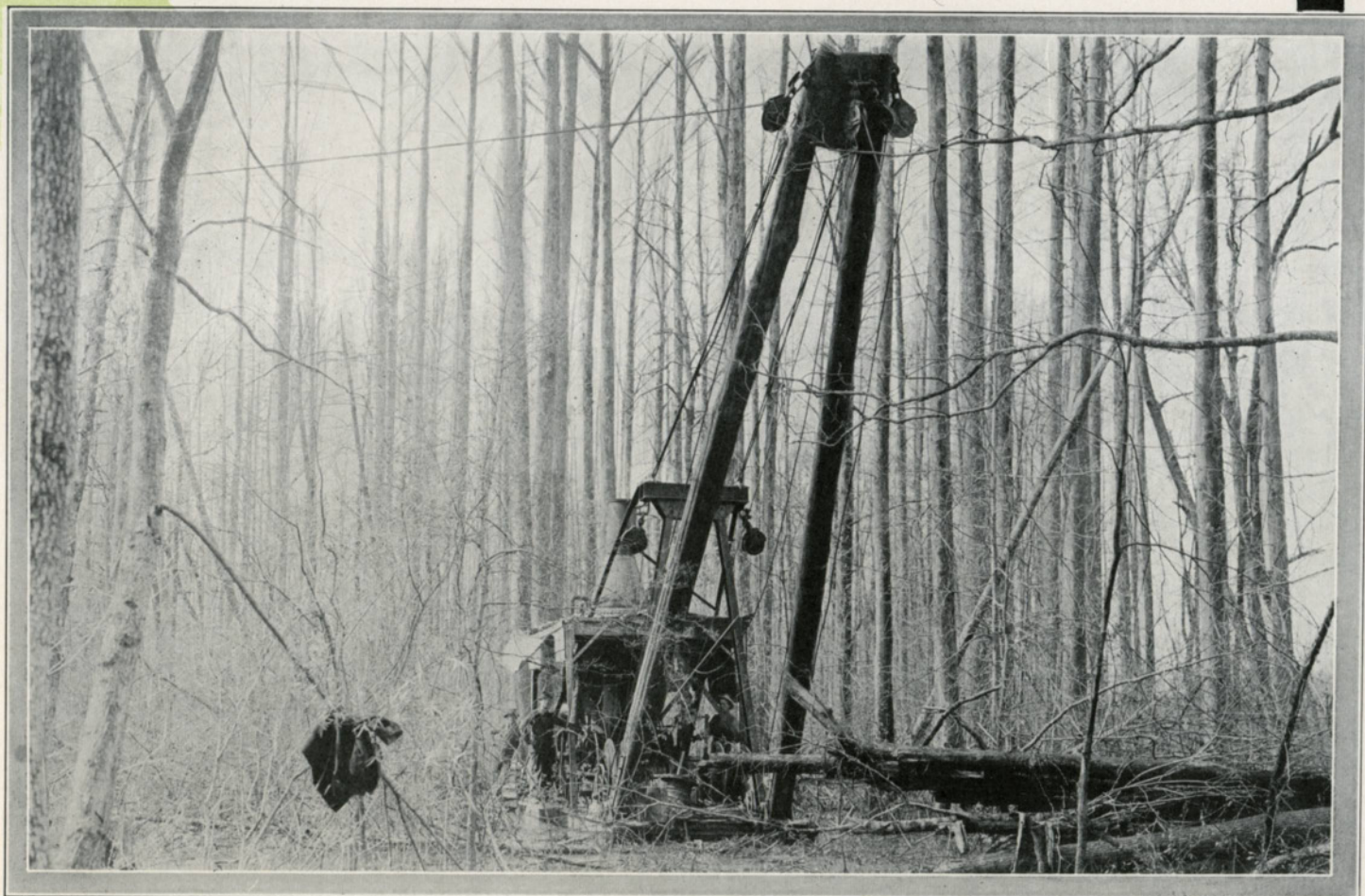
Clyde "Rapid" Ground Skidder Operating One Skid- ding Line with Cable Outhaul.
