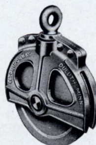
Clyde Loading block with cast steel housing and cast steel sheave with oil cellar for self lubrication.
