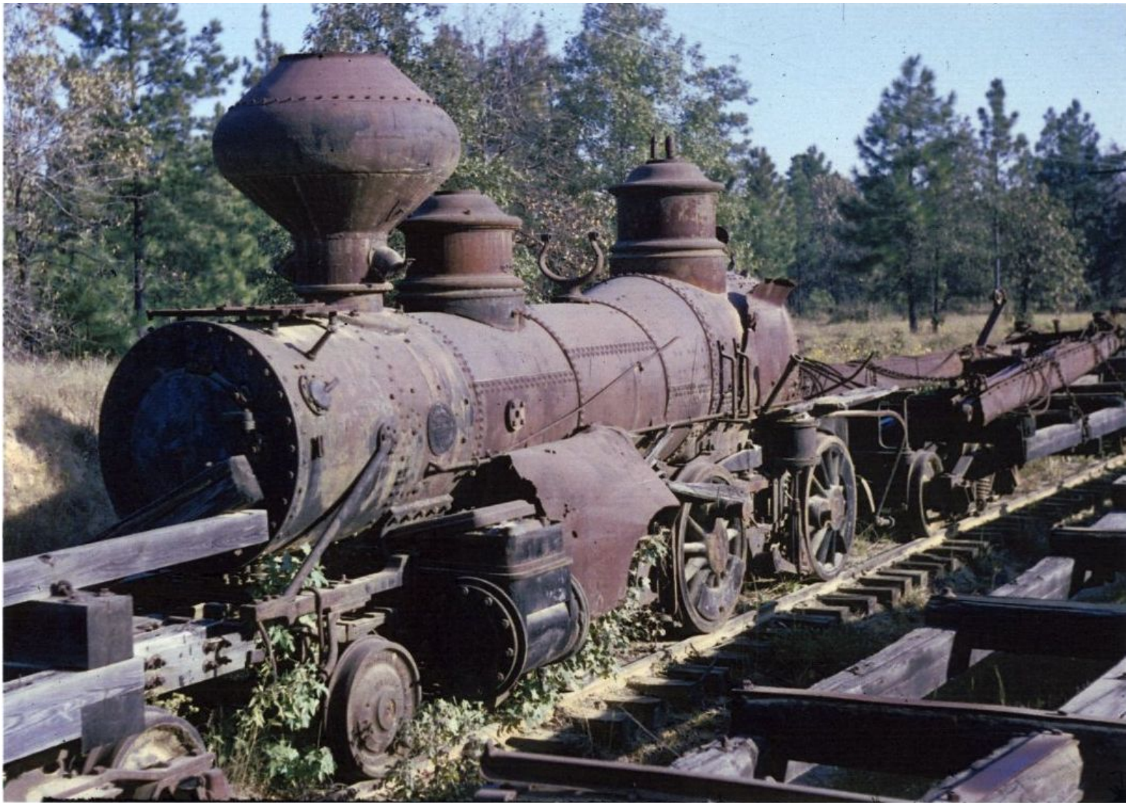
File #: NFma.H0671RSb, Date taken: 10/10/53, Long Leaf, LA. Credit: Gordon S. Crowell Photo: .. Baldwin 2-6-2. Built 1882. Builder's Number 6257
