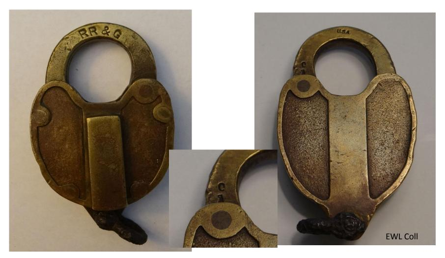
This is an RR&G type 2 lock. It maker is unknown, but its use is not. The enlargement of the rear of the shackle clearly shows the letter C and the number 1. This is a car lock. The number 1 may indicate that its key matches the keys for the type 1 lock, which they do. This suggests that the type 1 lock is a car lock as well. It is also, along with its keys, stamped RR&G, like the type 1 lock, not RR&G RR.
