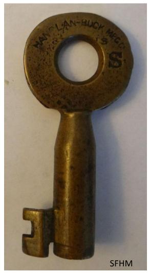
This is a switch key for the Handlan-Buck lock on the preceding page. Most of the known keys for these locks are stamped with a number 4, in addition to the letter S for Switch thus the identification of this lock and key set as type 4. Like all RR&G switch keys, they are stamped RR&G RR.
