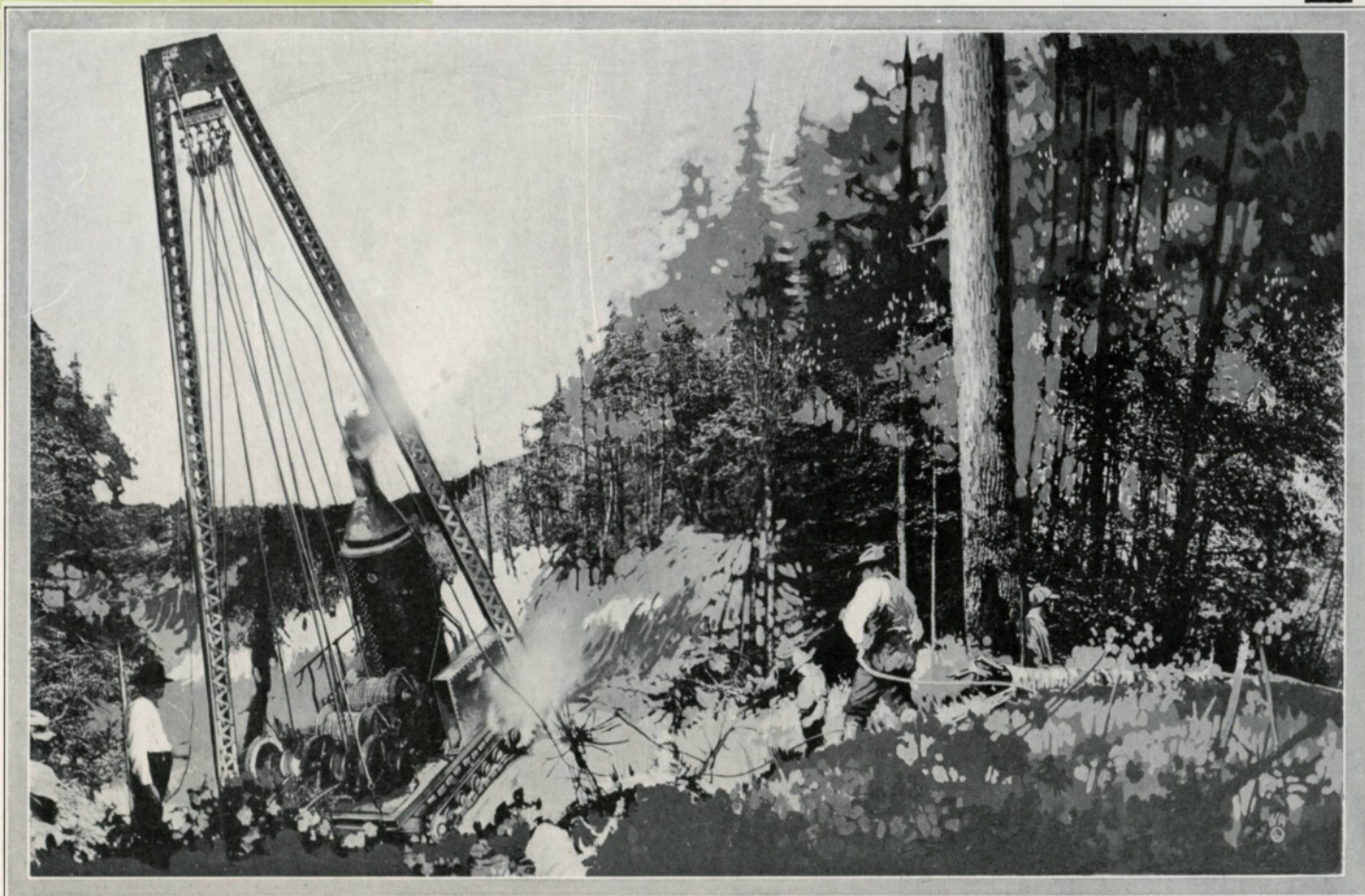
Clyde Traction Skidder Climbing Over Fifty Per Cent Grade.
