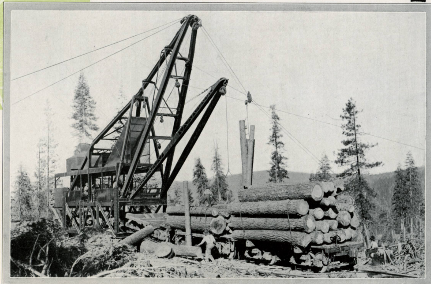
Clyde Universal Cableway Skidder and Loader (Heavy Type).
