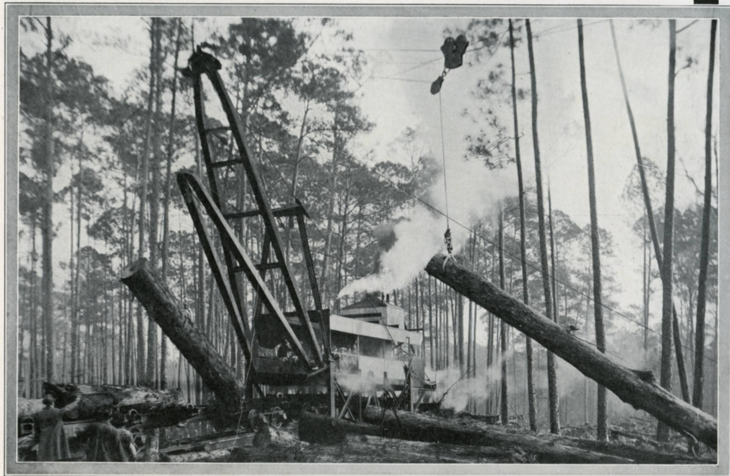
Clyde Universal Cableway Skidder and Loader (Light Type).
