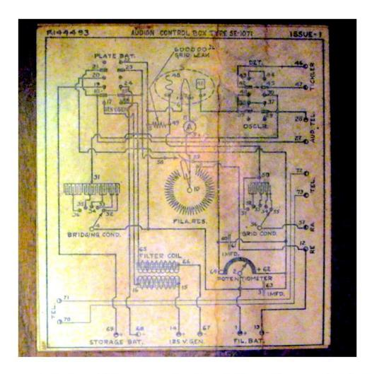
Note, top right, a connection for a tickler coil, suggesting that the IP-501 and its vacuum tube accessory made up a regenerative receiver. Along with its big antennas, that could explain some of the success of NDB.
