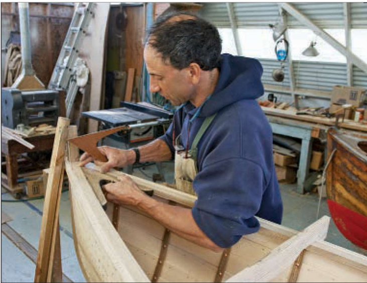
Top left —Fisher-Smith used Port Orford cedar planking, Oregon white oak frames, and a purpleheart inner keel in constructing KOHLENBERG's hull. Left —Careful attention to proportion, fit, and detailing pay homage to the aesthetics of the original VIKING. Above —A doorskin pattern has been used to mark the breasthook's shape on a just-right grown crook of Oregon white oak.
