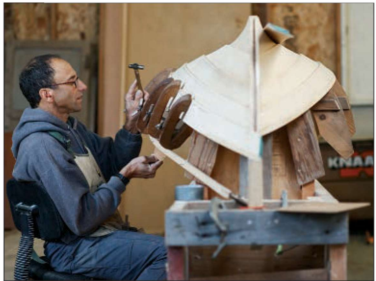
Above —By shaping patterns for each strake, Fisher-Smith made efficient use of his planking stock. Top right —For Fisher-Smith, lapstrake hull construction is all about carefully fitted planks; “they are key,” he says. Right —KOHLENBERG was built over the same molds used 23 years earlier for the construction of THOR.
