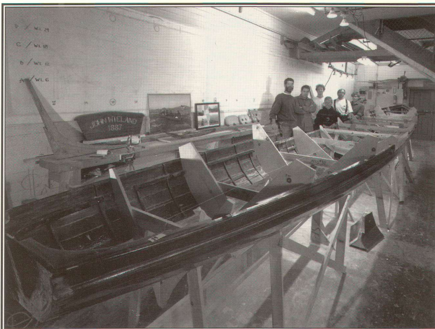
Early in the restoration process in the spring of 1994, most of the original planks and ribs are still in place, and the molds are in position. The lofting of the vessel can be seen on the shop wall behind the volunteers.
