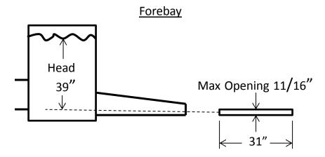
From the table in Appendix B, a head of 39 inches provides a discharge of 3.77 cubic feet per minute through a one inch by one inch orifice. The maximum area of our opening is 11/16" times 31 inches, or 21.313 square inches. This multiplied by 3.77 gives 80.348 cubic feet per minute, or 601 gallons per minute.
