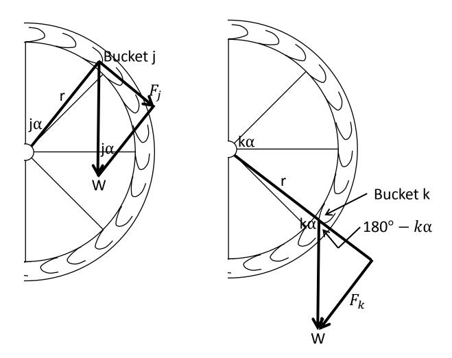
In this method, the water wheel is assumed to be stationary, and each bucket contains an amount of water of weight W. The torque contributed by each bucket is calculated, and the total torque T is the sum of all the individual torques contributed by the buckets.
