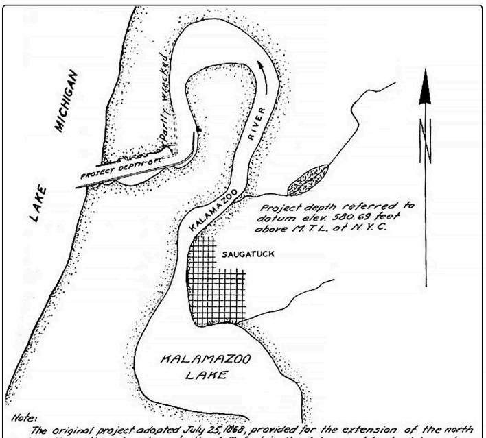
and south existing piers to a depth of 12 feet in the lake; and for dredging a chan--nel of the same depth between the piers and extending up the river as for as deep water near the first bend. This project with modifications of 1870 and 1882, providing for protection of the river banks and reduction of project depth to 8 feet, was not completed.
