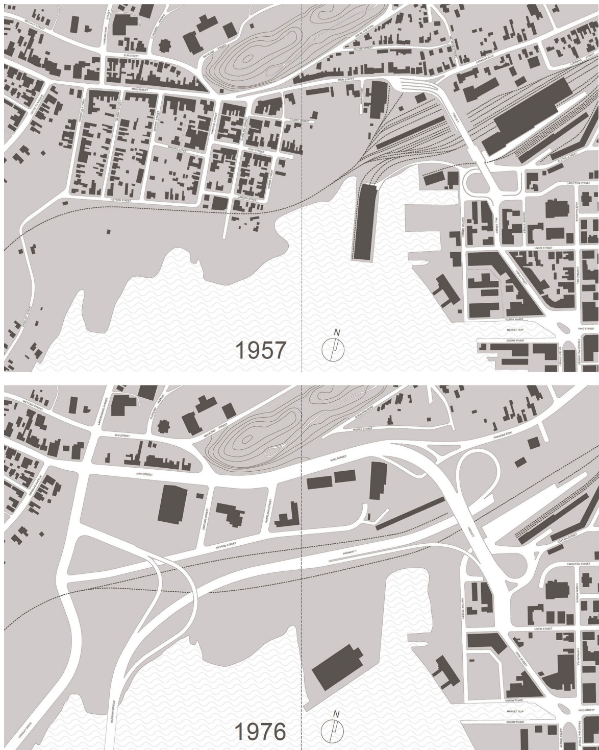
Figure 79: Figure-ground plan diagram of Saint John's Main Street-North End neighbourhood before (top - 1957) and after (bottom - 1976) the 1960s Urban renewal demolitions and bridge/highway construction.
