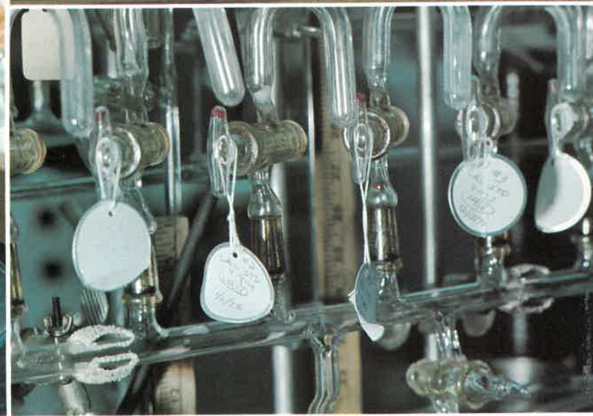
Vials, above, contain fractions of crude oil separated for gas chromatography. Tubes, below, contain carbon dioxide generated by oxidation during the identification process.
