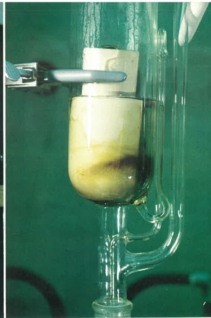
A Soxhlet Extractor isolates oily components from beach tar samples.
