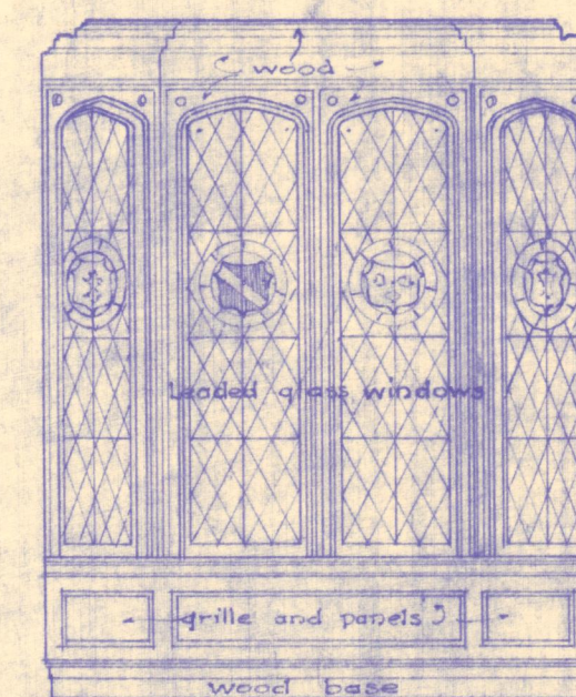
ELEVATION DAY WINDOW MAIN STAIR LANDING
