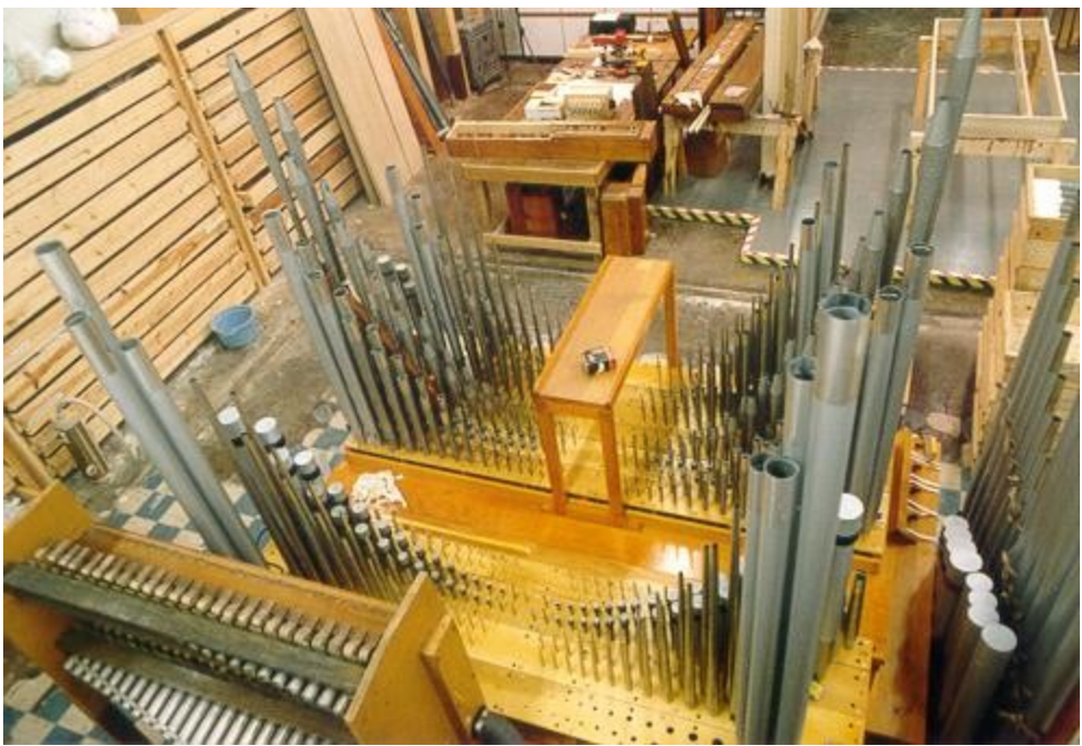
Above: CHOIR DIVISION, Francis Street First United Methodist Church, while erected in the shop of Quimby Pipe Organs, Inc., in 1996, prior to being dismantled for shipment and installation in the church. This section of the organ has 11 ranks or 618 pipes. The larger bass pipes are “offset” to the right from the main windchests. In the lower left is the “Harp”, with its graduated nickel-plated resonators and large piano-like hammers, which strike tuned metal bars.
