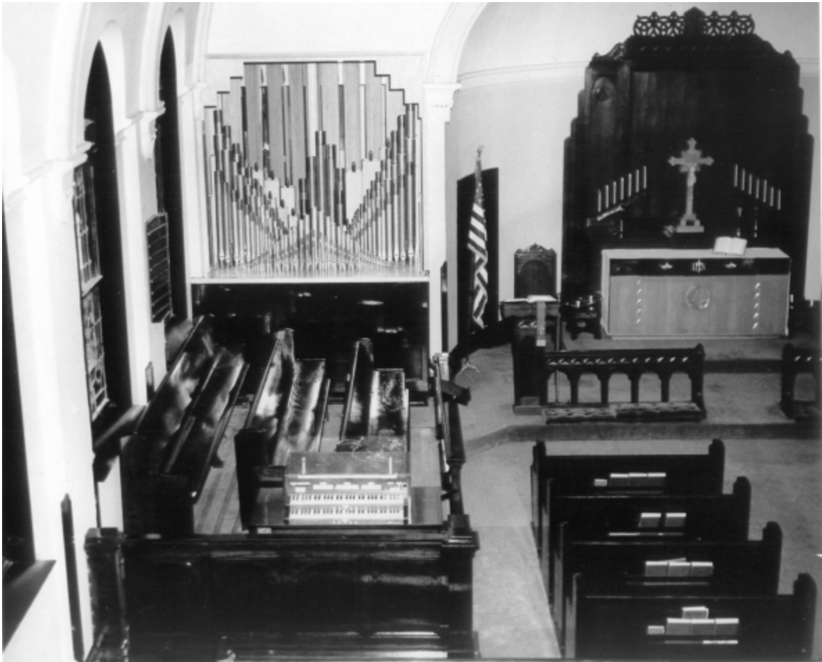
Original Wicks organ installation in St. Paul Lutheran Church, 14th & Lafayette, March 1956. The exposed pipes of the Great and Pedal divisions are now located behind a screened wall in the present building. The vertical louvers behind the pipework are called "swell shades" and open and close to control the volume of the Swell division.
