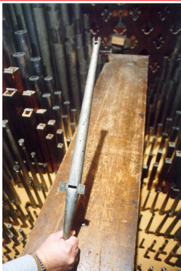
"Bell Gamba" pipe from one of the original Great division stops, so named because it tapers toward the top and then flares out at the end, called a "bell", like the flared end of some horn instruments. This is an unusual stop, with tonal characteristics
