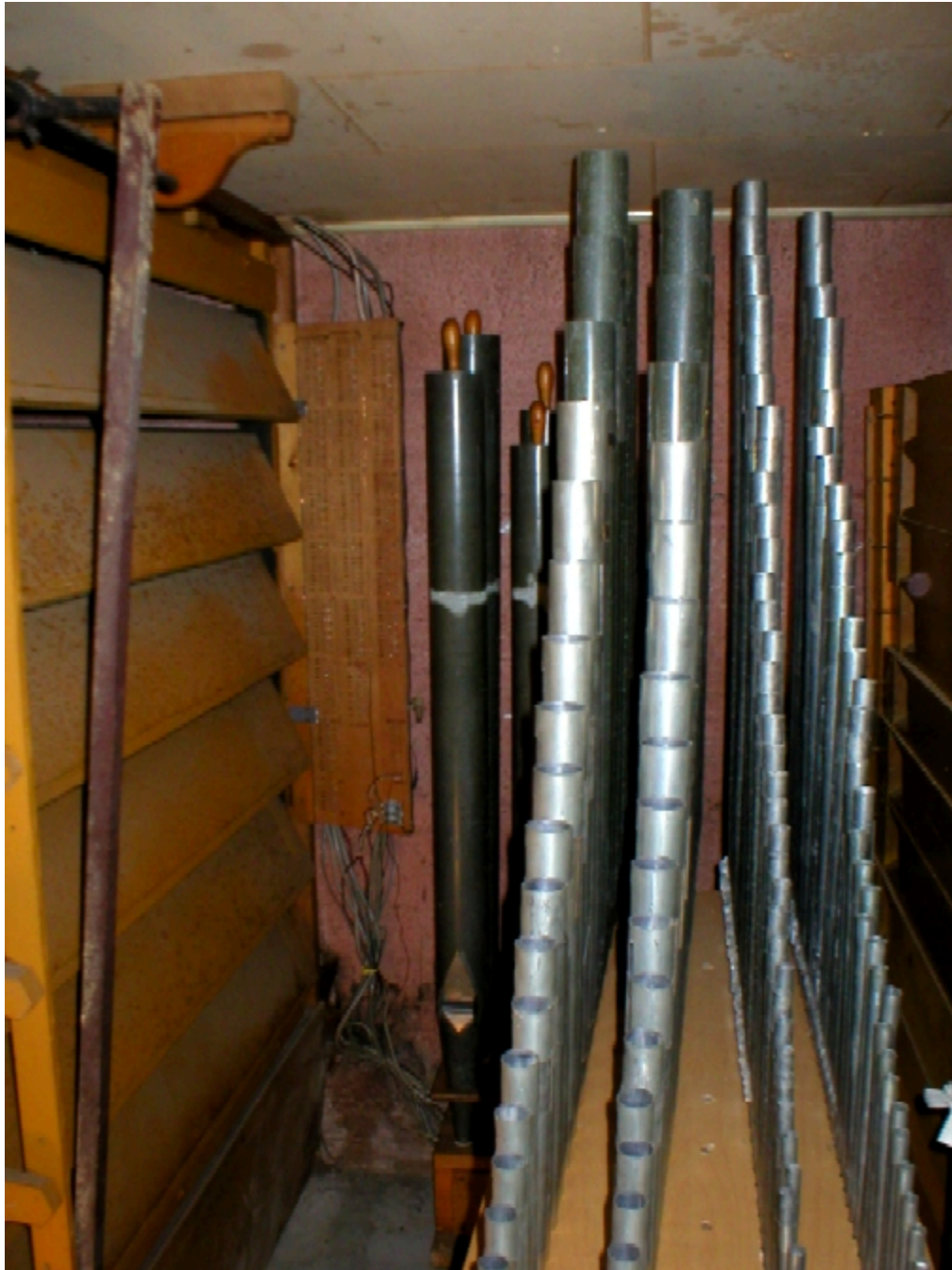
ORGAN CHAMBER located in the basement of the Clark-Sampson Funeral Home. The volume of sound is regulated by the louvered "expression shades" on the left side and is projected through a floor grate in the organ room above which contains the console.
