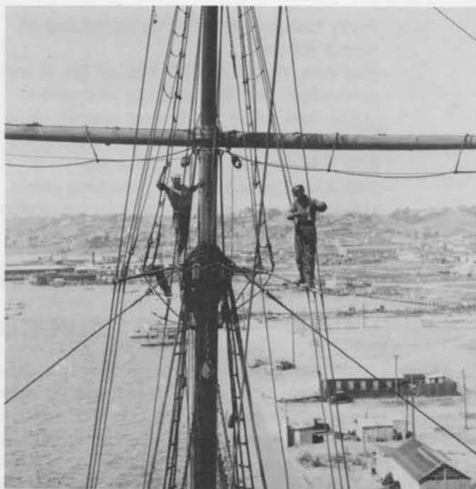
Photographed from the mainmast, two men work on the INDIA's rigging at her fore crosstrees. The fellow on the left is identified as "MacDonald," the one on the right as "Lebesque." The date is 1928, the place San Diego. Maritime Museum file photo
