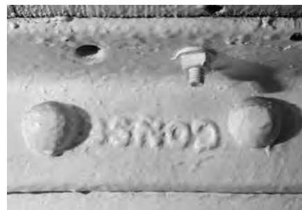
This "CONSETT" mark appears beneath the 'tweendeck on frame 23.
