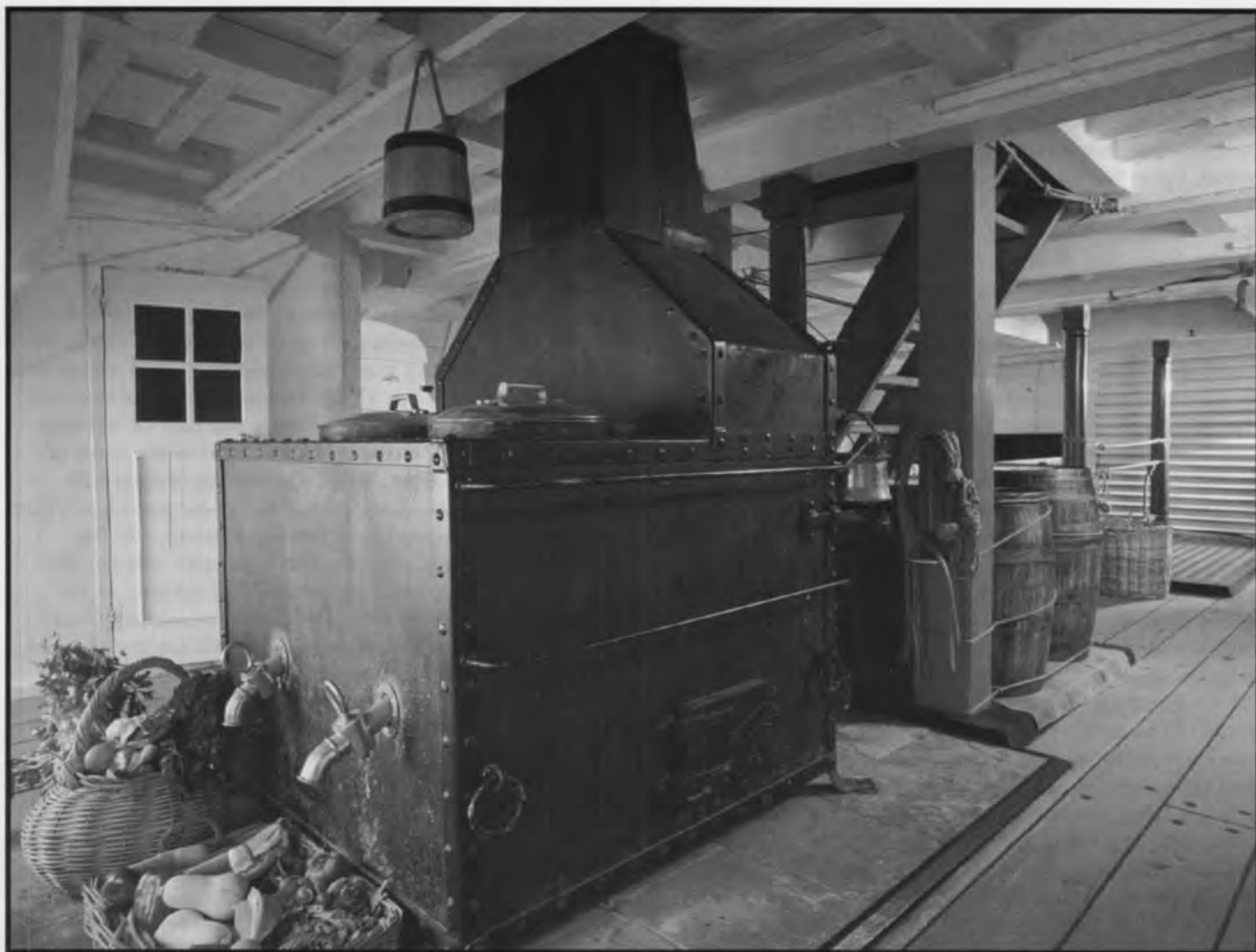
The large iron firehearth (stove) on which all the meals were cooked, installed in forward end of crew's mess decks. Doors to left (forward) lead to the cabins and storerooms for Captain Cook's boatswain, John Gathrey, and the carpenter, John Satterley. (Courtesy HM Bark Endeavour Foundation).
