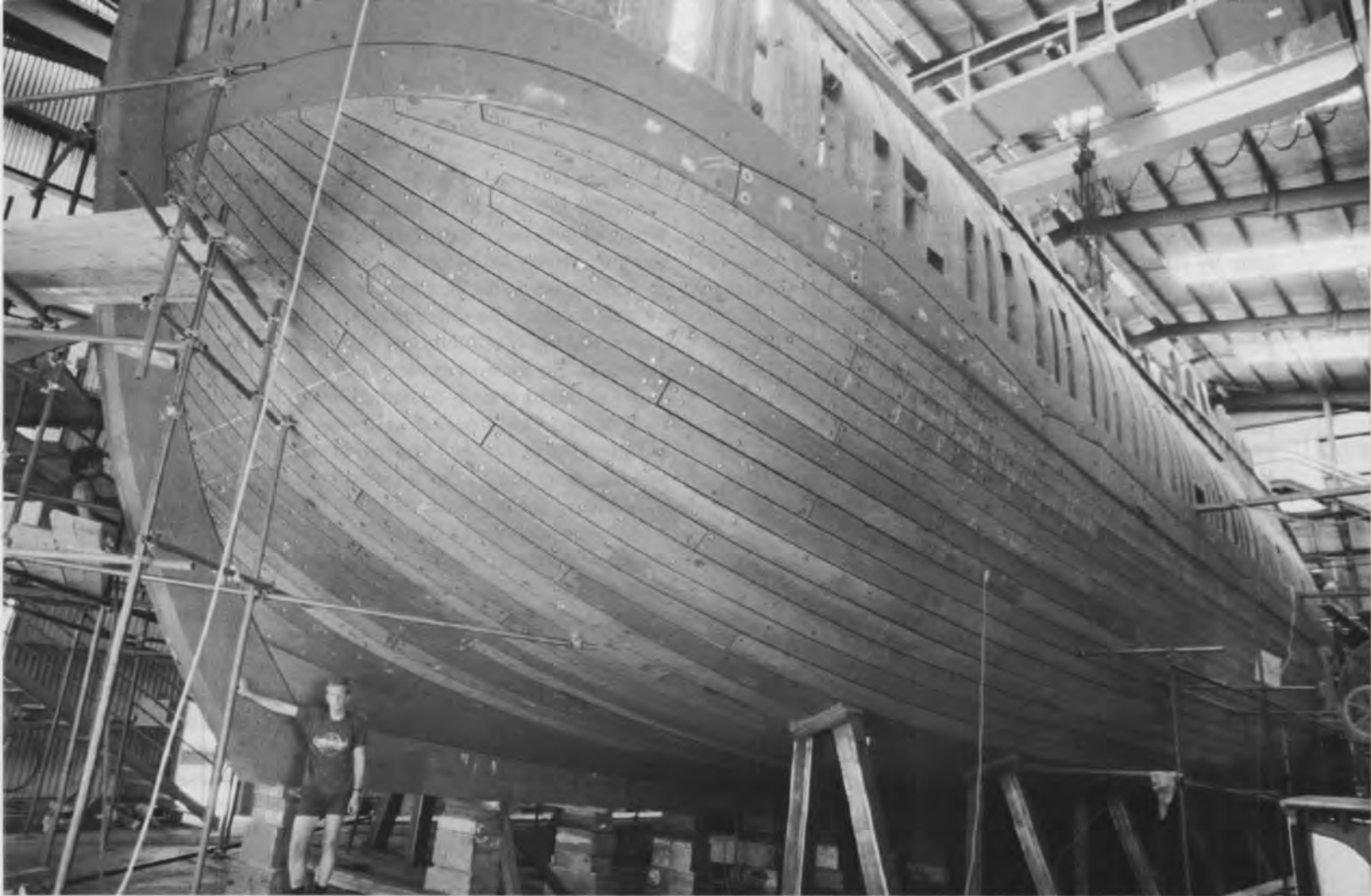
The massive lower stem dwarfs a workman posing below the hull of the Endeavour replica. Her bottom planking has been attached up to the level of the wales. (Courtesy HM Bark Endeavour Foundation).
