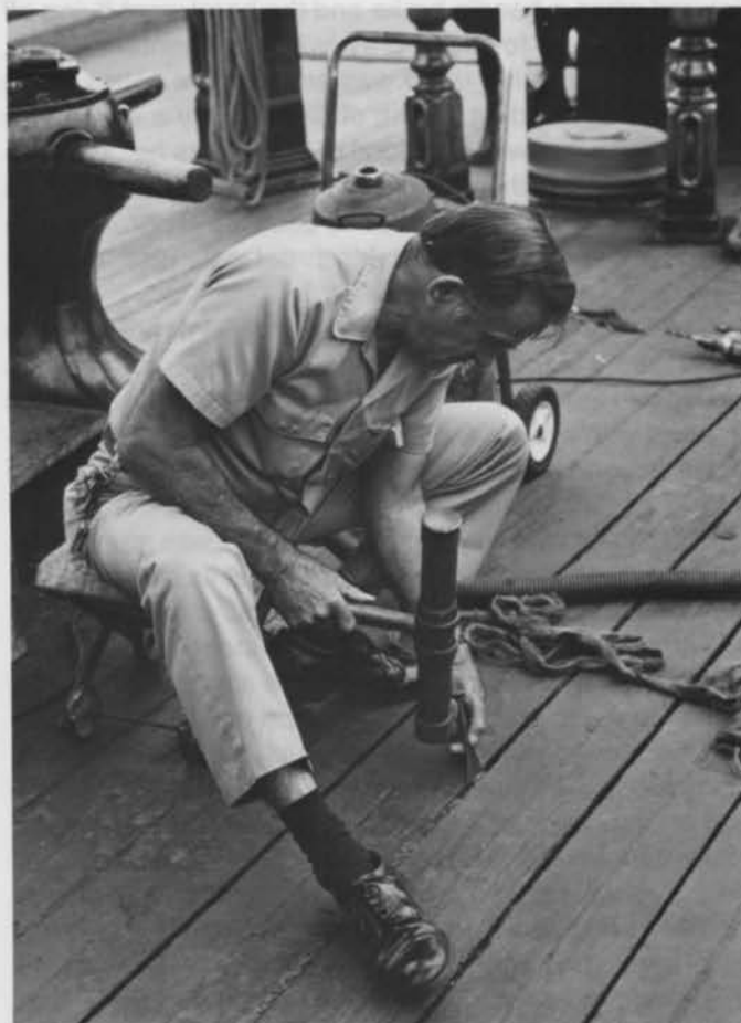
Museum maintenance chief Fred Krone caulks a deck seam in STAR OF INDIA. Today this work is carried on much as it has been for centuries.
