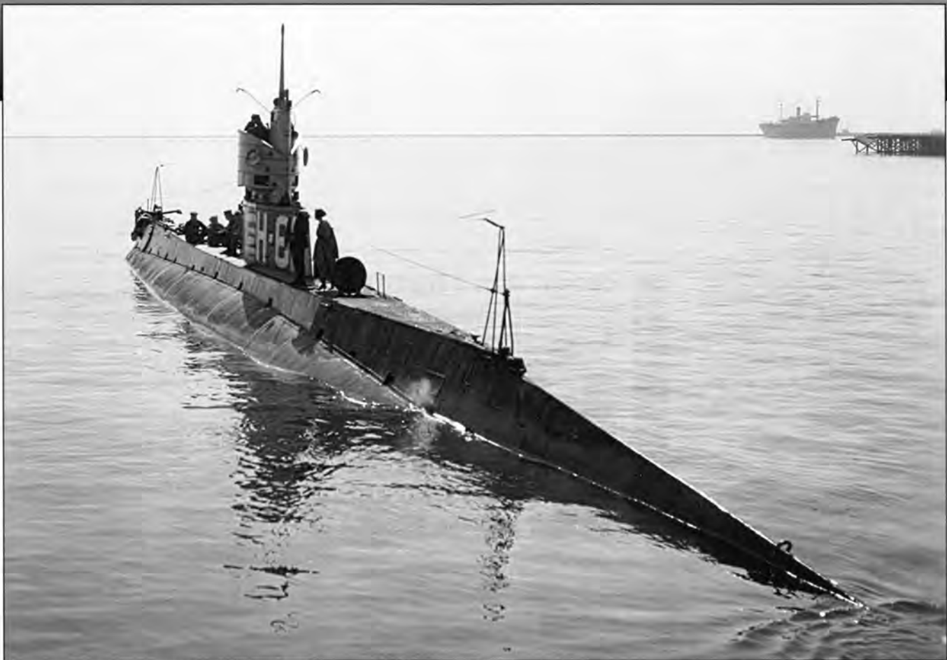
Pictured is H-6 in San Pedro on a calm day. The H-class shared many of the same characteristics as the F-class, but provided a “chariot” bridge and improvements in ventilation and periscopes.
