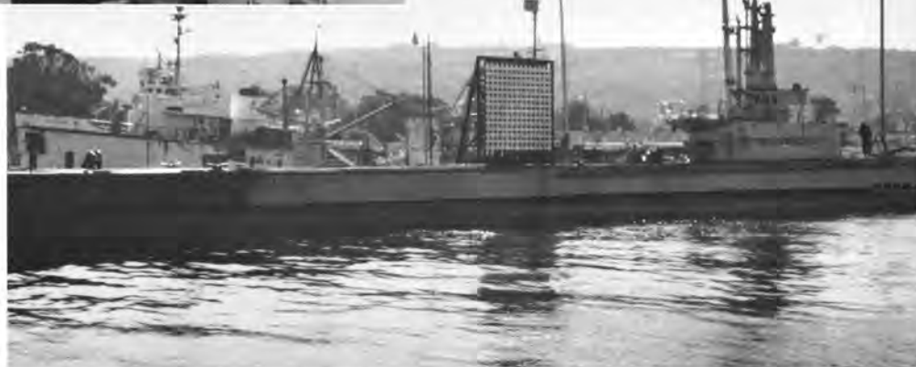
Below: Long Range Active Detection (LORAD) sonar array on deck of Baya berthed at waterfront area of U.S. Navy Electronics Laboratory in June 1955.
