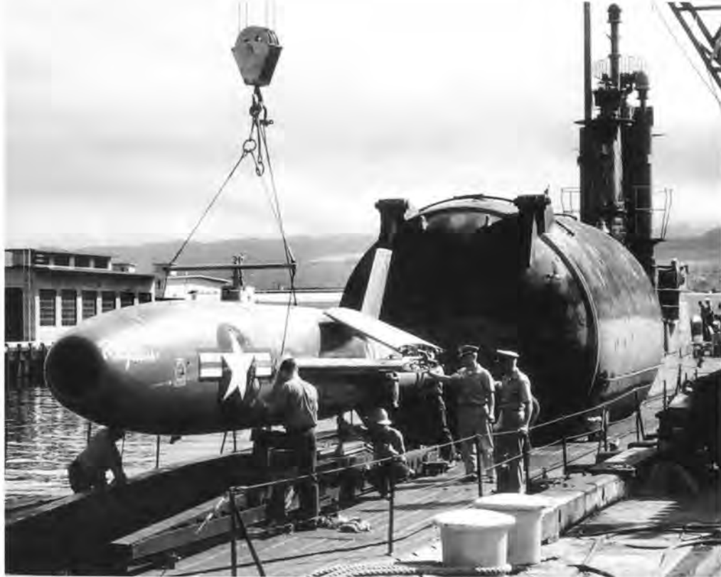
The Regulus missile is loaded aboard the Barbero (SSG-317), circa 1960. The crane has the missile positioned just in front of the container where it can be inspected before further loading.
