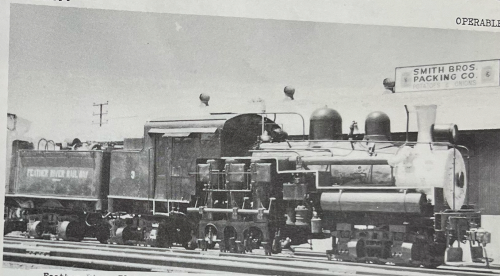
Feather River Rly. Shay No. 3 at Ferris, Cal., May 1967. Shay is now in San Diego at Santa Fe's 22nd Street Yard. Line shafts have been removed. (Eric Sanders)
