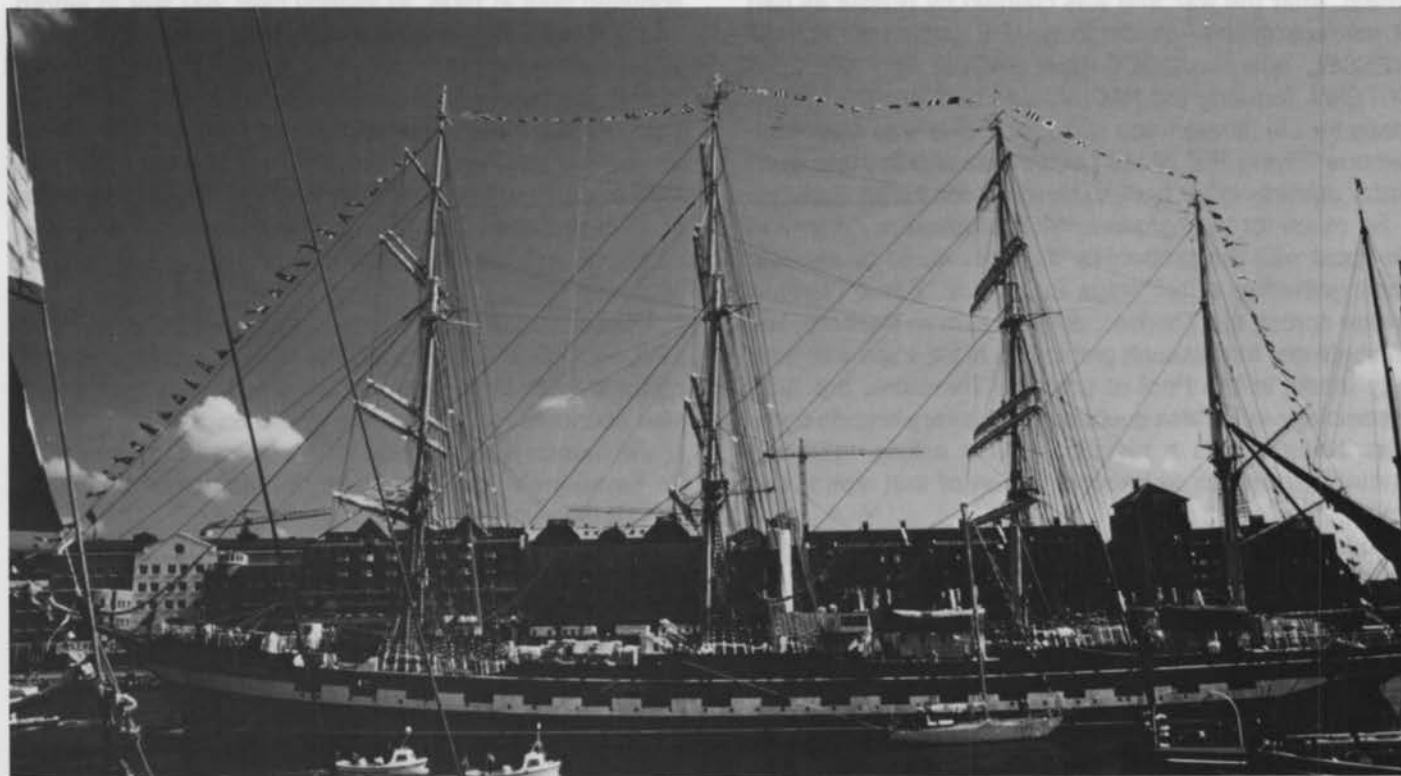
KRUZENSHTERN, the magnificent four-masted bark now under the Russian colors, formerly the German PADUA of the Flying P line. At 375.5 feet LOA and 3545 gross tons, she is a superb survivor of the great nitrate fleet that once
