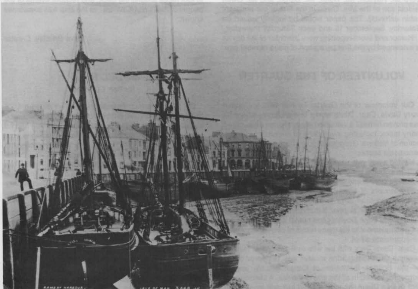
Ramsey Harbour, Isle of Man, about 1875. The two vessels in the foreground are topsail schooners, of the basic type designed to come to rest on an even keel when the tide goes out, as here. The schooner on the left is the ARIEL
