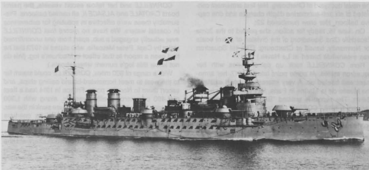
One of the many powerful French warships in World War I was VICTOR HUGO, an armored cruiser with 7.6-inch guns and torpedo tubes. Note such distinctive French
