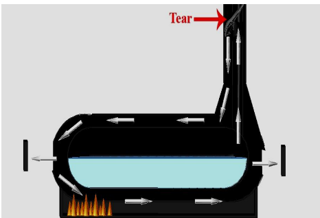
Diagram illustrating how the Jenny Lind boiler blew , spewing steam, and killing or injuring many passengers.
