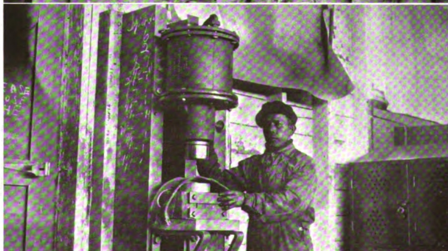
(Top) Power saw for splitting scrap air hose. (Middle) Hose after being split, ready for steaming. (Bottom) Air press equipped with die for stamping gaskets.
