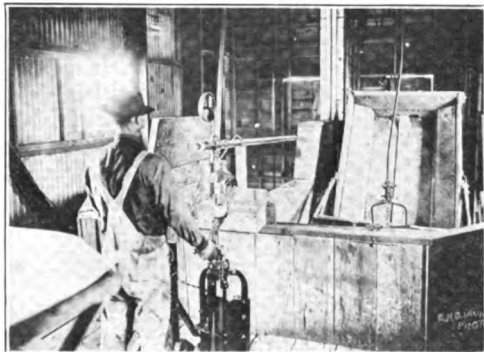
Hoist Operator Located in Tippie Tower Handling Three-Way Brake Air Valve with Right Hand and Controller with Left Hand. The Dumped Mine Car Is Shown on the Right.
