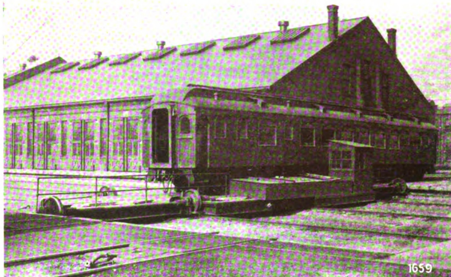
WHITING ONE-MOTOR ELECTRIC TRANSFER TABLE Capacity 80 Tons. Length 74 ft. 10 in. The Pullman Co., Buffalo, N. Y.
