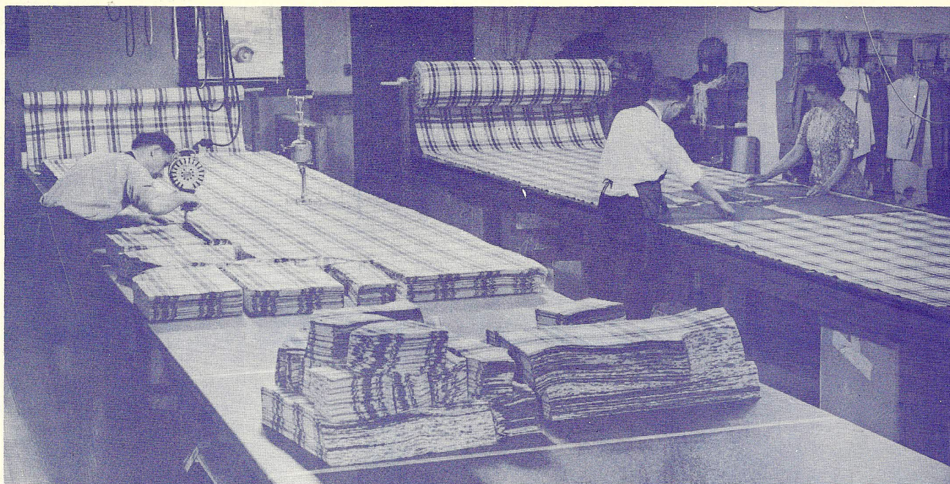
This machine cuts many layers of fabric in a single operation.
