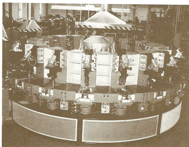
18 station Desma polyurethane injection machine
