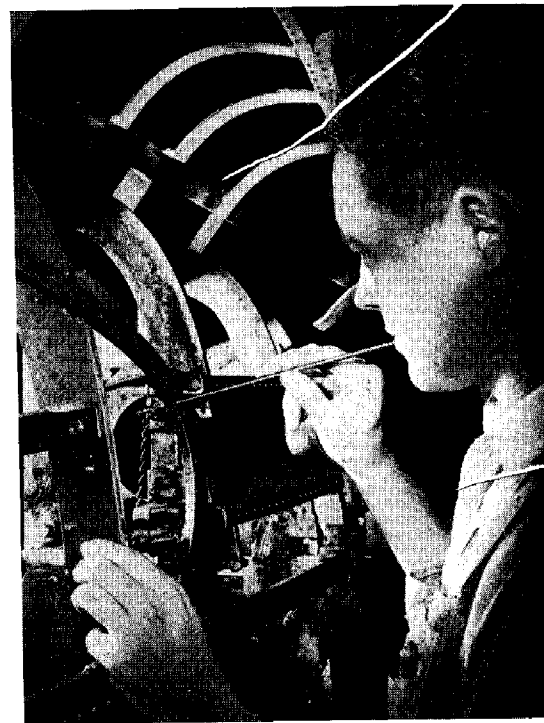
CHECKING tooling before use, as Carl Hofer is doing above, has helped cut down Dept. 89's drill breakage greatly.
