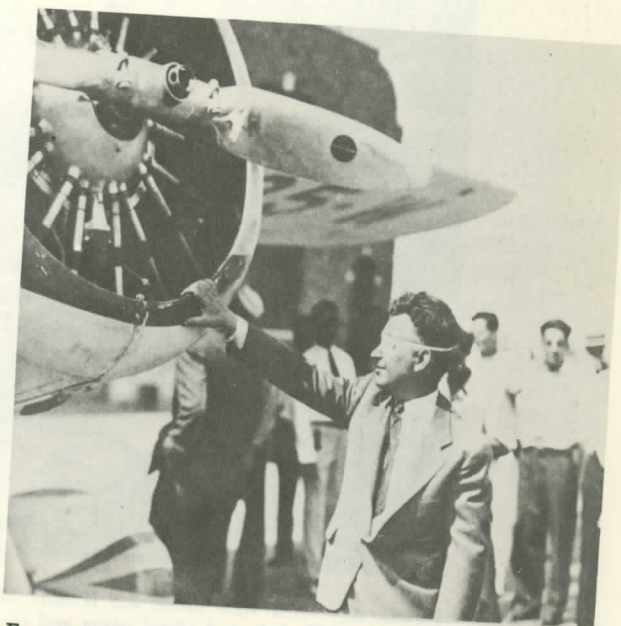
FIGURE 64.—Post examines the Winnie Mae at Floyd Bennett Airfield, New York, after completion of the 1933 solo world flight. The lower cowling reveals the dents placed there in the Flat, Alaska, nose over. The propeller is the fixed-pitch Hamilton Standard substituted at Flat for the controllable pitch propeller damaged in the nose over. (Courtesy Pratt and Whitney Aircraft.)
