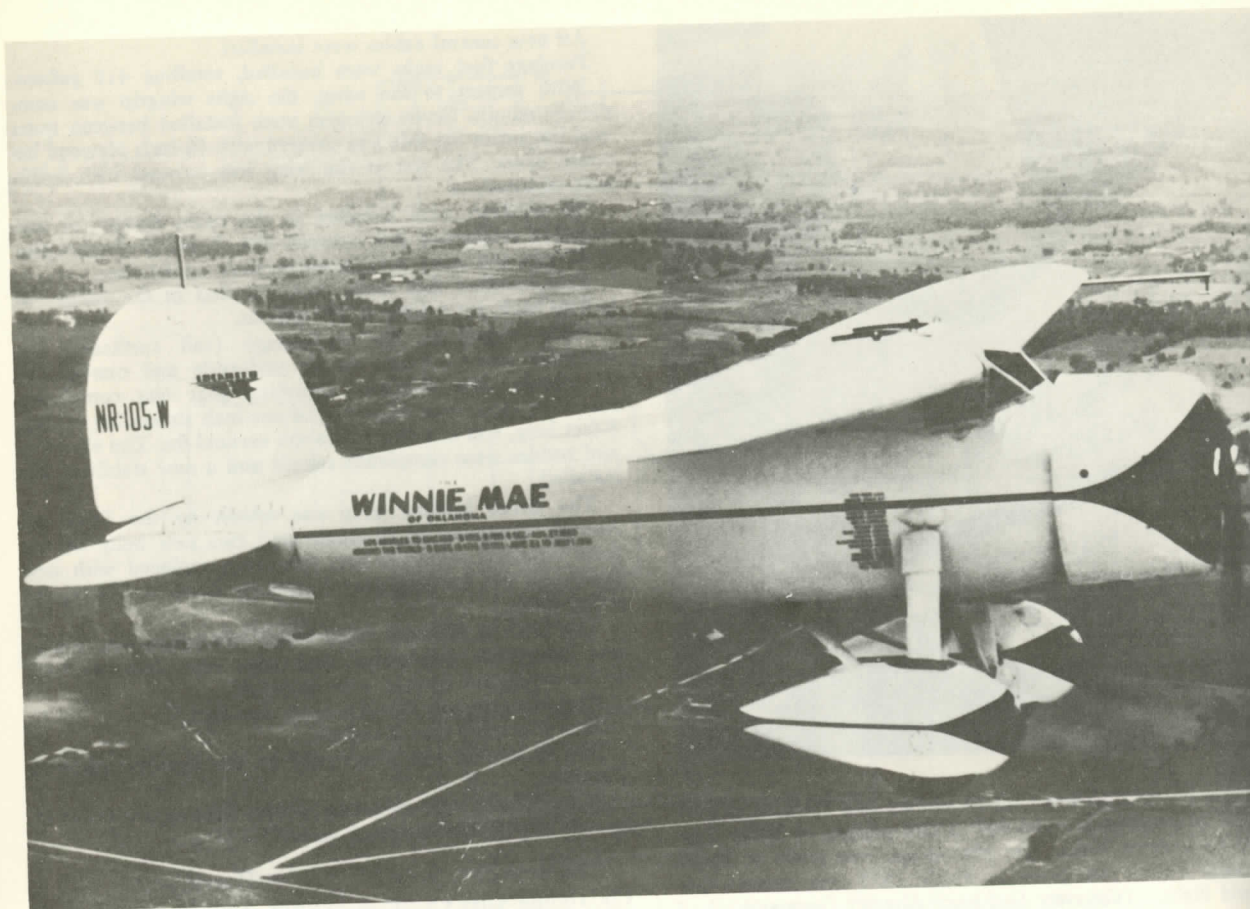
FIGURE 55.—The Winnie Mae is shown ready for the around-the-world solo record flight attempt. The “sense” antenna post on the fin is clearly evident. (Courtesy Jimmy Gerschler and Smithsonian Institution.)
