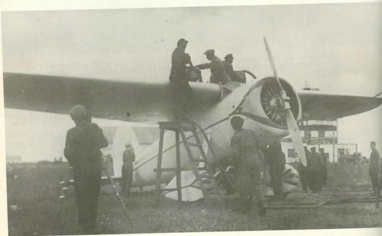
FIGURE 58.—A crew of Russians energetically and efficiently refuel the Winnie Mae at Novosibirsk on July 18, 1933. Note that the left- and right-wing tanks are being filled through chamois cloths to remove any contaminating water. A photographer in the left foreground records the event. Post stated that he got excellent service in Russia and received a very warm welcome at each stop, including Moscow, the preceding stop, where he made an unscheduled landing. The Chief of Transaviation, Mr. A. Petrov, requested the chief of the West Siberian Administration and the chief of the Far Eastern Administration to give full assistance to Fay Gillis and Wiley Post regarding the flight. (Courtesy Fay Gillis Wells.)
