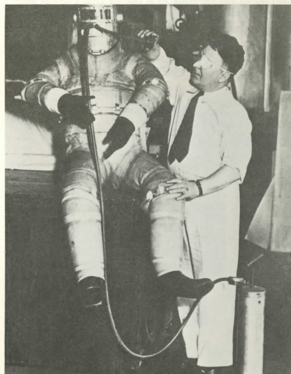
FIGURE 72.—Wiley Post's second pressure suit is shown during a static pressure test at the B. F. Goodrich Company in Akron, Ohio. This pressure suit was the first to employ flexible elbow and knee points. The suit was entered through the waist, which was sealed with two large metal plates held together with wing nuts. The oxygen was brought in just below the visor. Post had to be cut out of the suit when he became stuck in it. Photograph made in July 1934. (Courtesy Popular Mechanics Magazine.)
