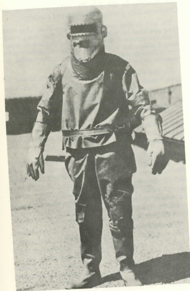
FIGURE 70.—Post's first full pressure suit and helmet. This suit was made of rubberized parachute fabric. Earphone bulges are shown on the helmet. The rectangular plastic vision plate was replaced in the later version with a circular glass window. The metal belt sealed the top half of the suit to the bottom half, when the suit was pressurized. The suit was entered at the waist. Photograph taken on roof of B. F. Goodrich plant, Los Angeles, June 1934. (Courtesy 1935 Aircraft Year Book.)
