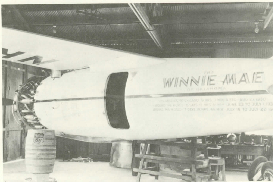
FIGURE 96.—The Winnie Mae is shown being prepared for a transcontinental stratosphere flight. This photograph was made in January 1935 at the original Lockheed hangar in Burbank. This hangar had been a "glass factory" prior to its use by Lockheed. The cowlings have been removed and cleaned of paint (seen on floor behind fuselage). The aircraft is suspended by pulleys from a ceiling beam by utilizing the hoist eye hooks on the upper wing. The belly-landing skid made of spruce has been glued in place and is now metal clad. Under the rear fuselage in the background on the workbench is the spherical container for the liquid oxygen. (Courtesy Phillips Petroleum.)
