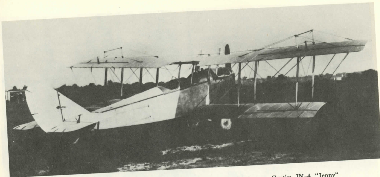
FIGURE 8.—The Curtiss "Canuck," Canadian version of the famous Curtiss JN-4 "Jenny" military training airplane of World War I, became a popular barnstorming airplane in the 1920s. The Canuck was typically powered by a Curtiss OX-5 engine of 90 horsepower, which gave the airplane a 60-mile per hour cruising speed with a 45-mile per hour stalling speed. The Canuck had ailerons on both wings, which gave it a more rapid roll rate than the American Jenny. The OX-5 engine was a water-cooled, eight-cylinder engine that consumed nine gallons of fuel per hour. The fuel tank capacity was 20 gallons. (Courtesy Smithsonian Institution.)
