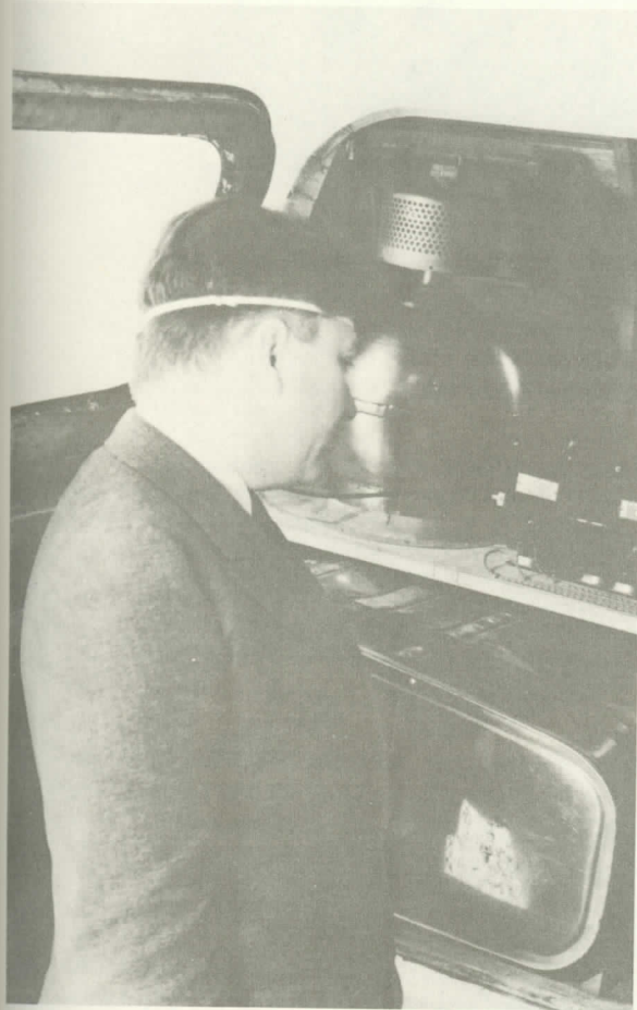
FIGURE 102.—Post views the liquid-oxygen container as stowed in the fuselage of the Winnie Mae in preparation for the long-distance stratosphere flights. Aft of the container is the Westport power supply for the radio compass. A fuselage fuel tank is mounted below the above equipment. (Courtesy Phillips Petroleum Co.)
