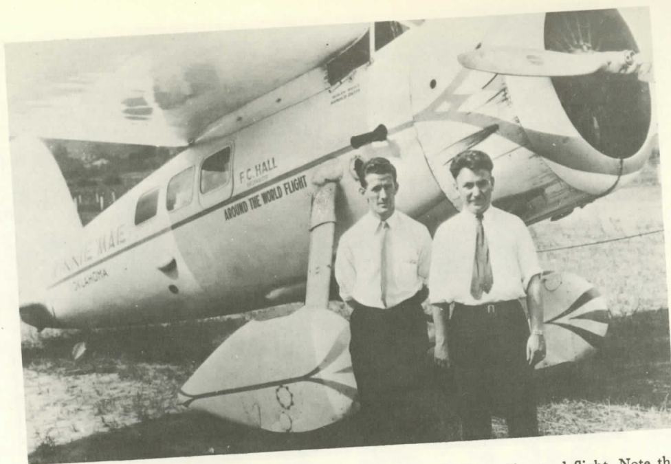
FIGURE 38.—Gatty and Post are seen after their 1931 around-the-world record flight. Note the oil-streaked cowling of the Winnie Mae . The small hole in the cowling above the trim is for the crank that spins the hand-inertial starter. The venturi tube just aft of the cowling above Gatty's head is for Gatty's duplicate set of gyroscopic flight instruments. The airscoop for cooling Post's feet is seen just above Gatty's right ear. The Pathé rooster emblem on the fuselage has been painted over but still shows slightly through. Gatty's drift and ground-speed instrument ports are shown under the rear windows. The propeller is a fixed-pitch Hamilton Standard. The right-wheel pant has a metal cover on top for a fuel-handler step. The attachment point to the wheel axel is shown with eight screws, while below this, the cover for the tire inflation valve is shown. The aircraft is roped off for protection. On this flight, Post confirmed his theory that the "variance in time" would disrupt his body biological rhythms and derogue flight performance. He was the first to publish on this phenomenon, which later became known as "circadian rhythm disruption." (Courtesy Lockheed Aircraft Company.)
