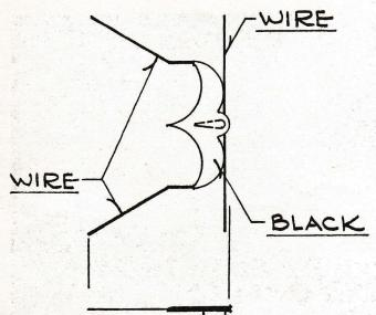
ALTERNATE ANTENNA-LOCATE TOP CENTER OF FUSELAGE AT TRAILING EDGE OF WING
