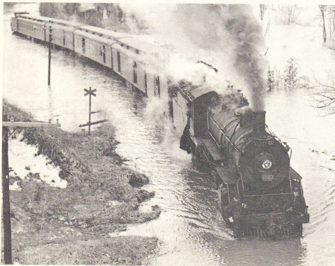
LEFT: Where diesels fear to tread, K-3-b 5583 wades through the floodwaters of Hurricane Hazel in the fall of 1954. Note the absence of an air reservoir on the pilot beam. /R. Buck Coll'n
