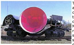
The Railroad Museum's latest acquisition is an INCO slag pot car, which in the past was used to move molten slag from the converters to the slag piles. Many Capreol residents remember going to the INCO site at night and watch the stream of red-hot slag rushing down the hill. The car, donated
