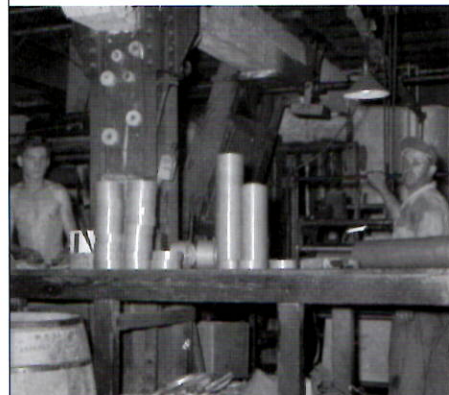
Slitting rolls of Tufftape® with the Kidder Slitter -- 1953 Photo
